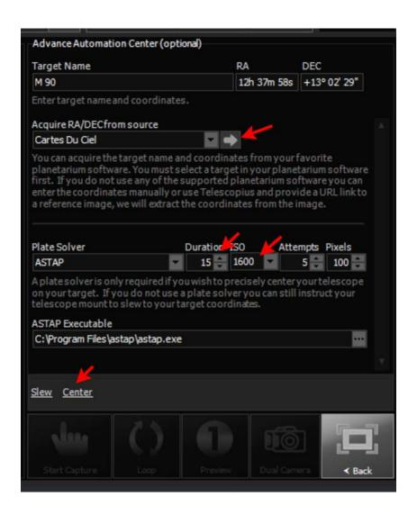
• Type in the coordinates of the object (R.A. and Dec., epoch of current date, *not* 2000) OR open Cartes du Ciel and find and select the object, then tell BackyardNikon/BackyardEOS to acquire the coordinates from Cartes du Ciel. (Do that by clicking on the arrow.) This will also put in its name.
